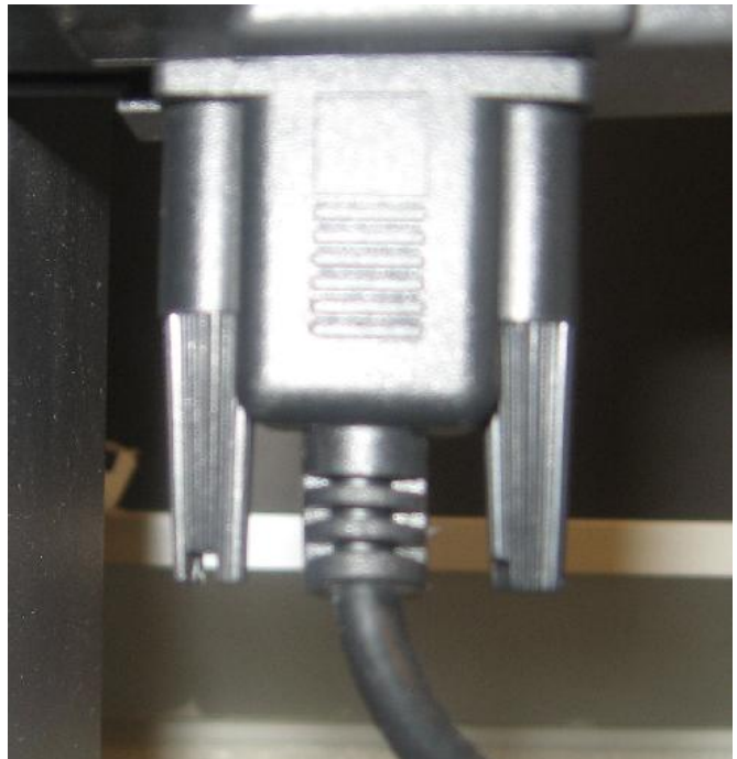
Serial end for cable that is used for an older model of Smartboard
